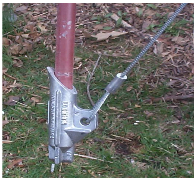
Drive Rod inserts into Anchor Head
