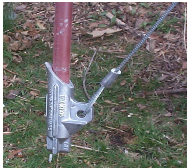
Drive Rod inserts into Anchor Head
